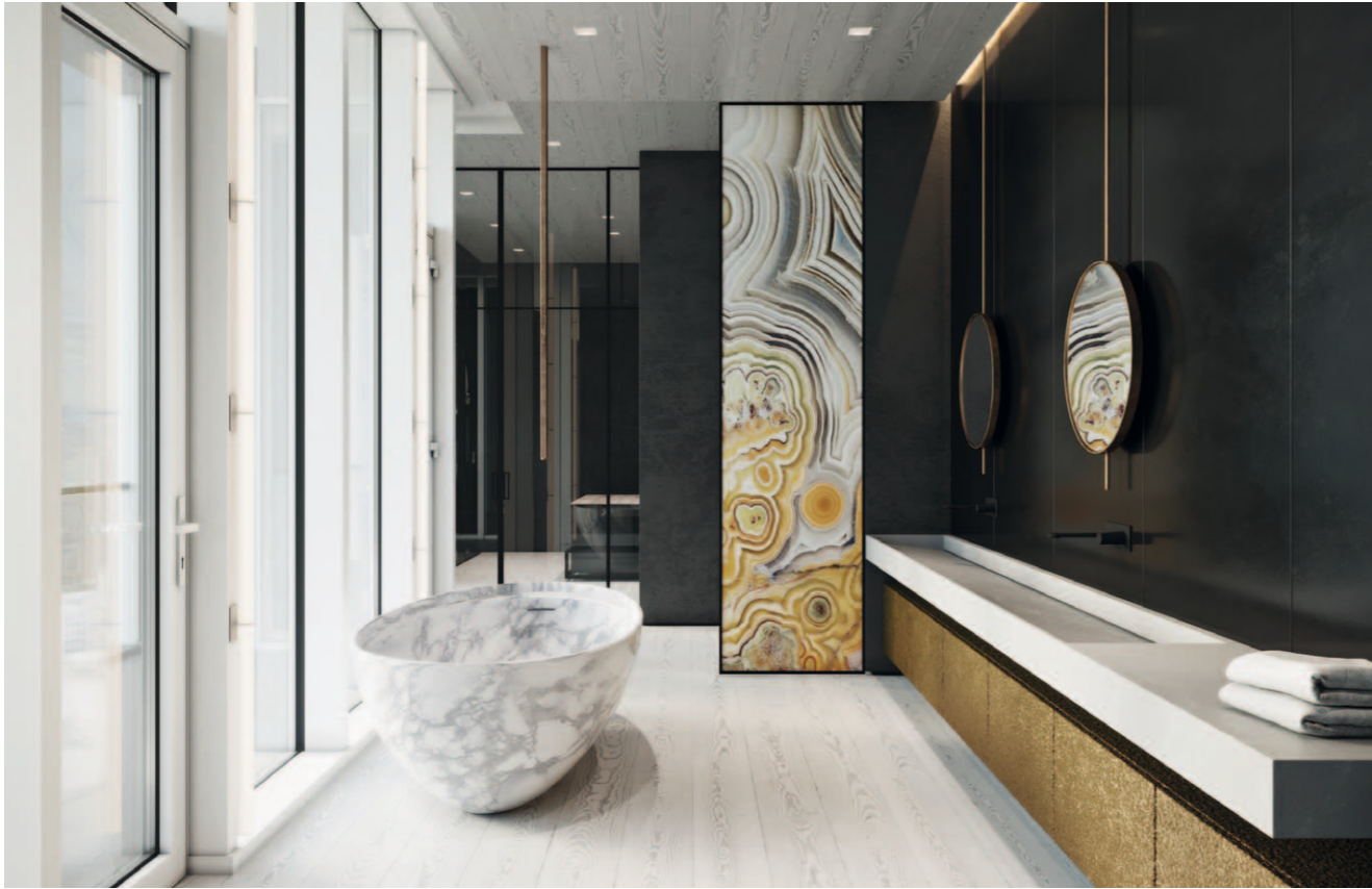
The master bathroom is lined with hot-rolled steel panels, floating monumental marble and hammered brass vanities, counterposed against a honey onyx divider. The bathtub was custom designed and fabricated from a single block of CNC-milled statuary white marble.
